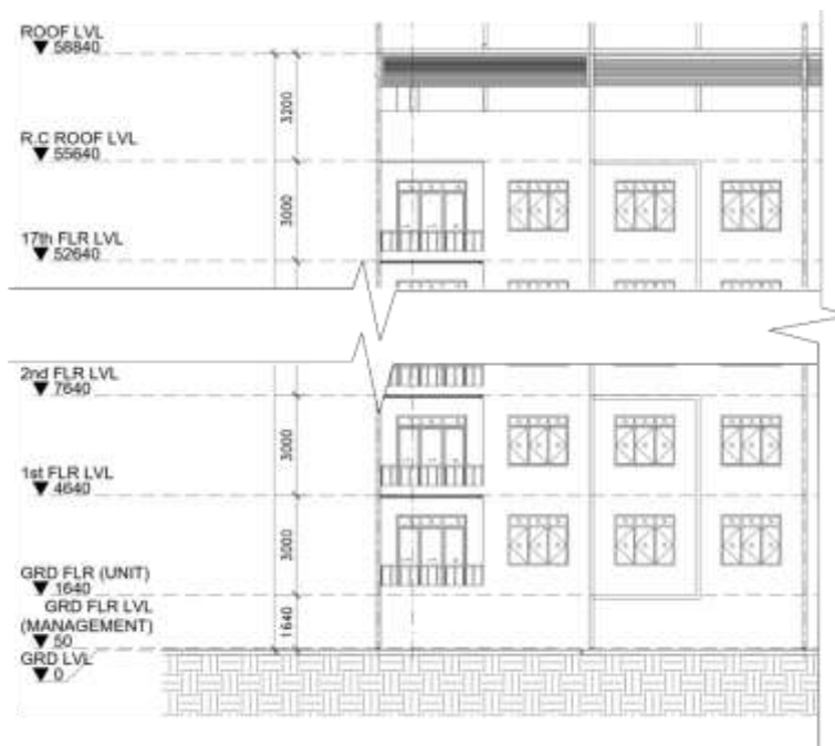
Figure 8. Typical Floor Height for 18-Storey Apartment
