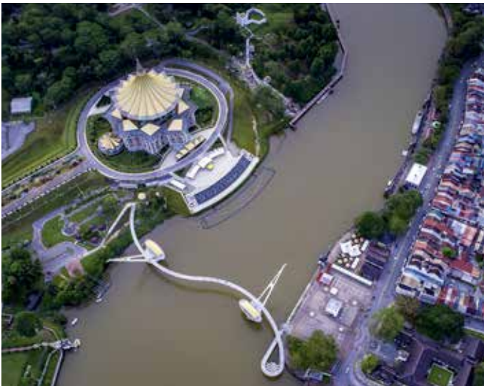
The bridge's steel spaceframe is suspended from two 50-metre-high steel towers that are angled steeply away from each other
