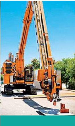
◀ 'Hadrian', the fully-automatic robotic bricklayer capable of building more than 150 homes annually, will be tested in Australian markets first before it is ready to be shipped abroad. ▶
