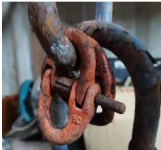
Figure 16: Corroded hoisting tackles
