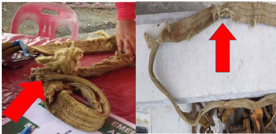
Figure 13: Defective hoisting webbing sling
