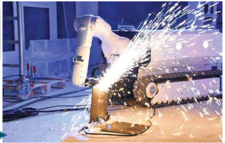
Precision cutting with the robot arm's plasma torch tool
