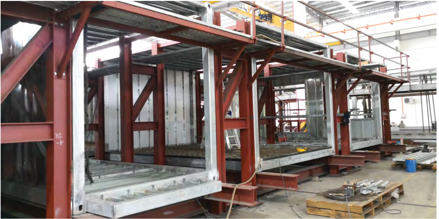
The 2D elements were designed to be assembled into 3D units in the transit factory
