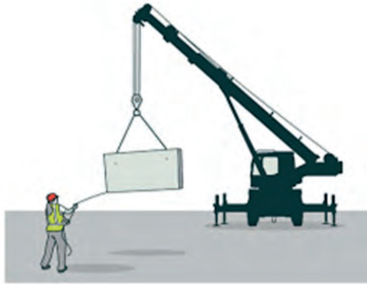
Figure 22. Lifting precast component
