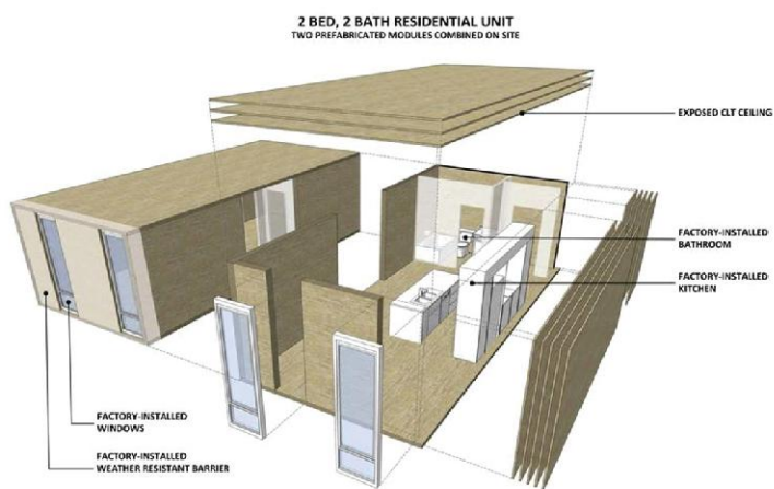
Figure 1.8. Example of a Timber VM
